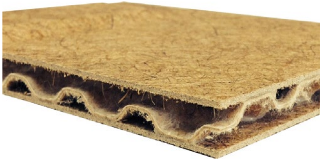
Another example of a sandwich moulded part
